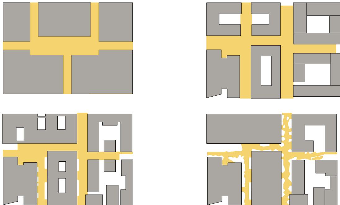
FIG 4.1 Plans showing evolution of public realm of Block 8. Top left: 2002 North Lotts masterplan Top right: 2014 SDZ masterplan Bottom left: 2015 masterplan Bottom right: Completed scheme, excluding landscaping. Source: Authors own
